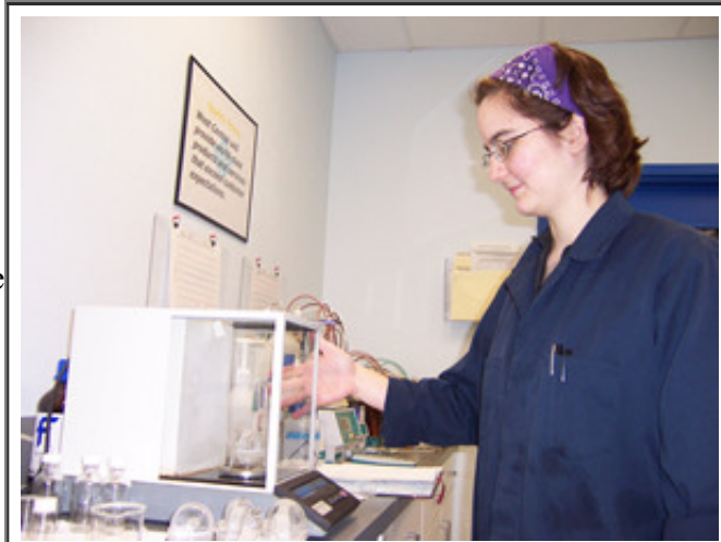
Laboratory technologist Megan Fry measures SoyChlor moisture, just one of West Central's daily quality-consistency checks.
